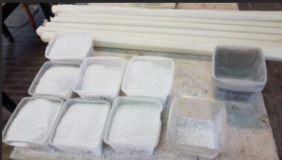
Glass powders ground to various particle sizes
