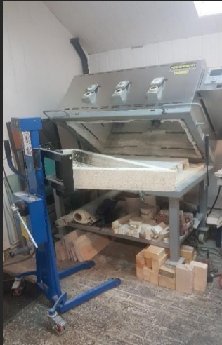
Nabatherm fusing kiln, for glass firing and annealing (the mold is first dewaxed in another kiln)
