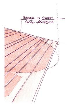
Bar-code Dehors is a platform made of Corten steel, a raw material that is extremely resistant and weatherproof. It features a warm brown surface made even more pleasant and uniform by a special beeswax treatment.
