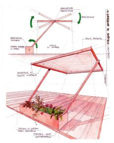
**Tagliasole** is the rectangular awning, ready to revolutionize the concept of shaded space. Made of Corten steel, it is intertwined with carbon or fibreglass threads, thus creating a large and pleasant shaded area for a number of outdoor settings.
