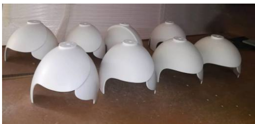
Corian® objects made of thermo-folding
