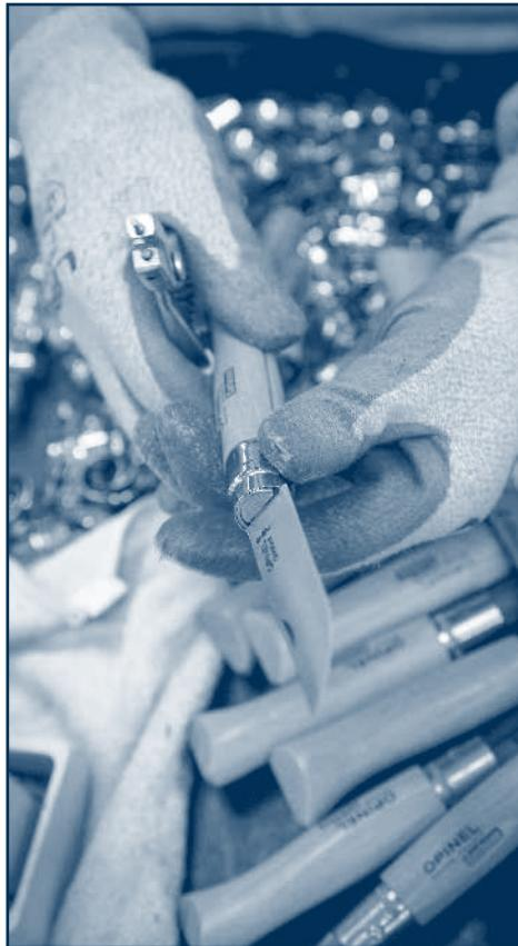
Assembling the knife combines several steps: putting together the handle, the blade and the fixed ring.
