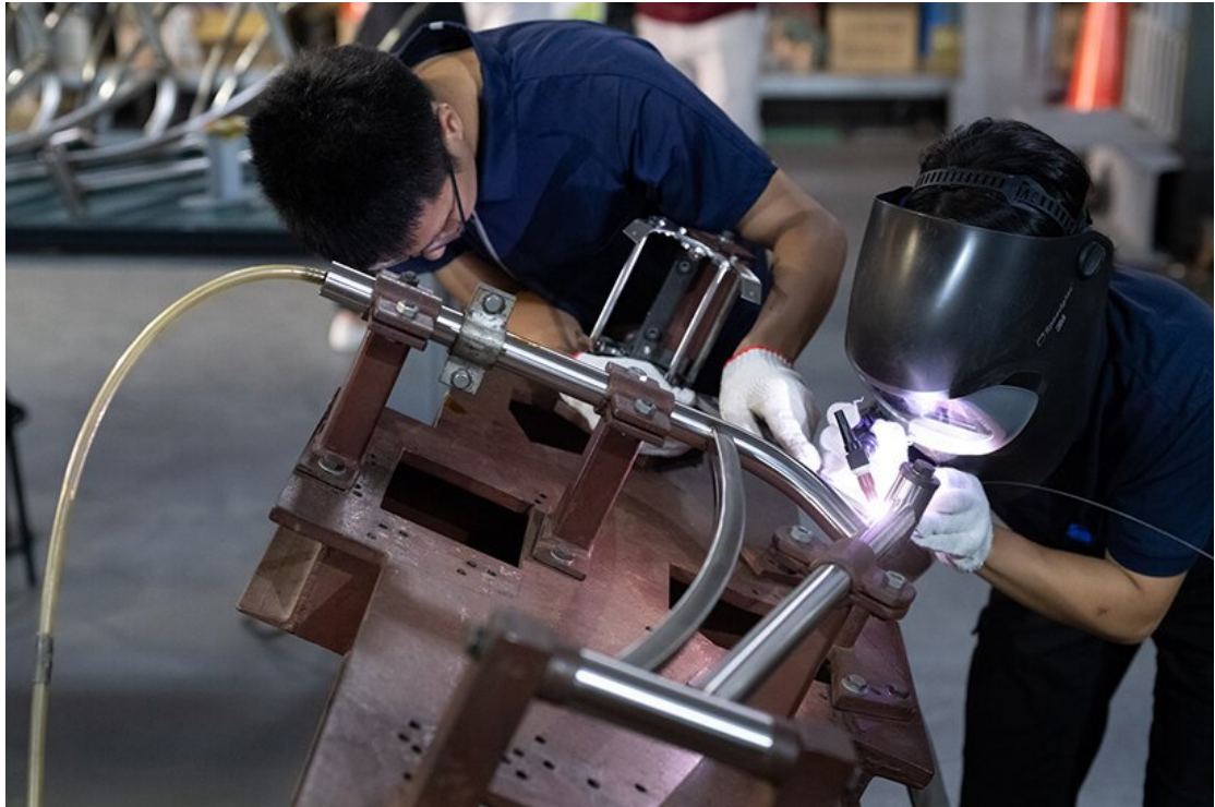
welding the distinct and strong frame of the bike
