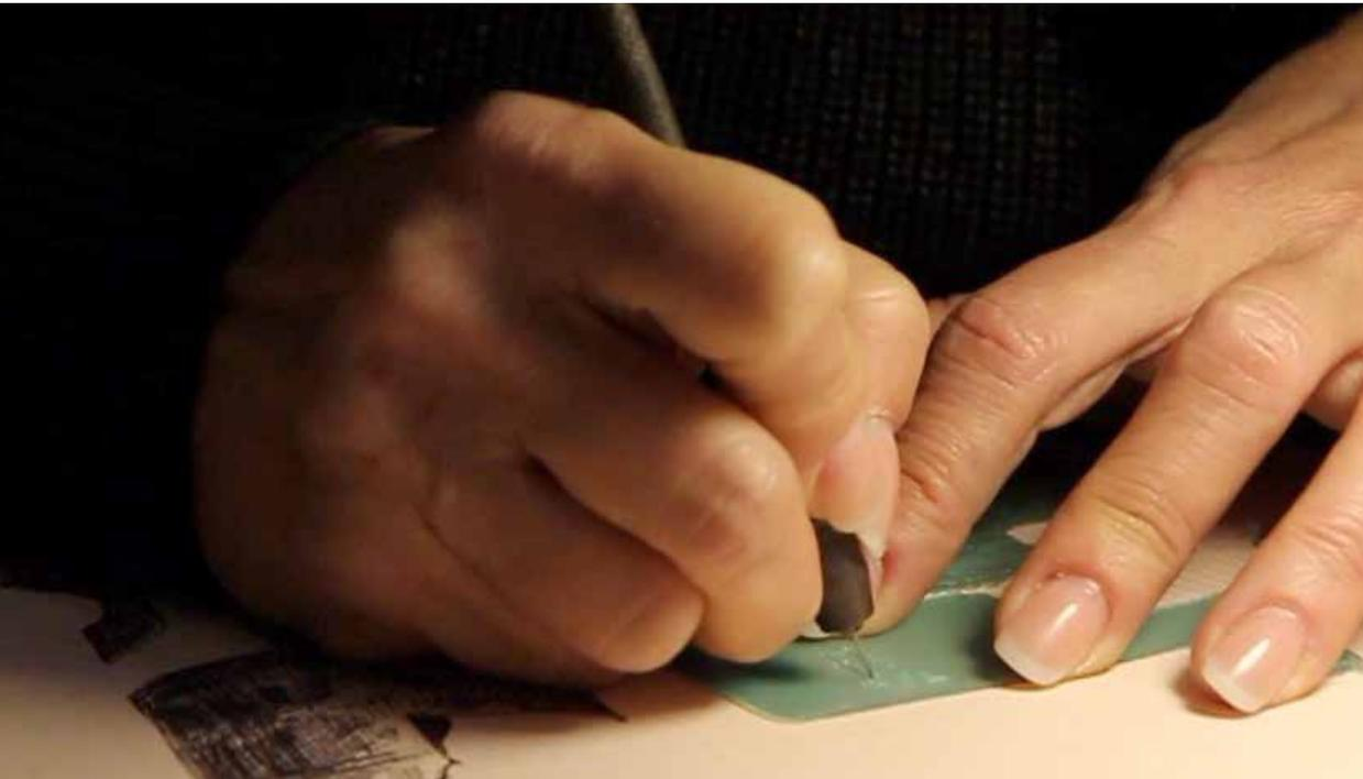
The procedure starts from the modeling of the wax in a micro-sculpture from which a plaster cast is obtained. The metal melts, slips into the shapes left empty by the wax called "lost" with heat and becomes a jewel.
