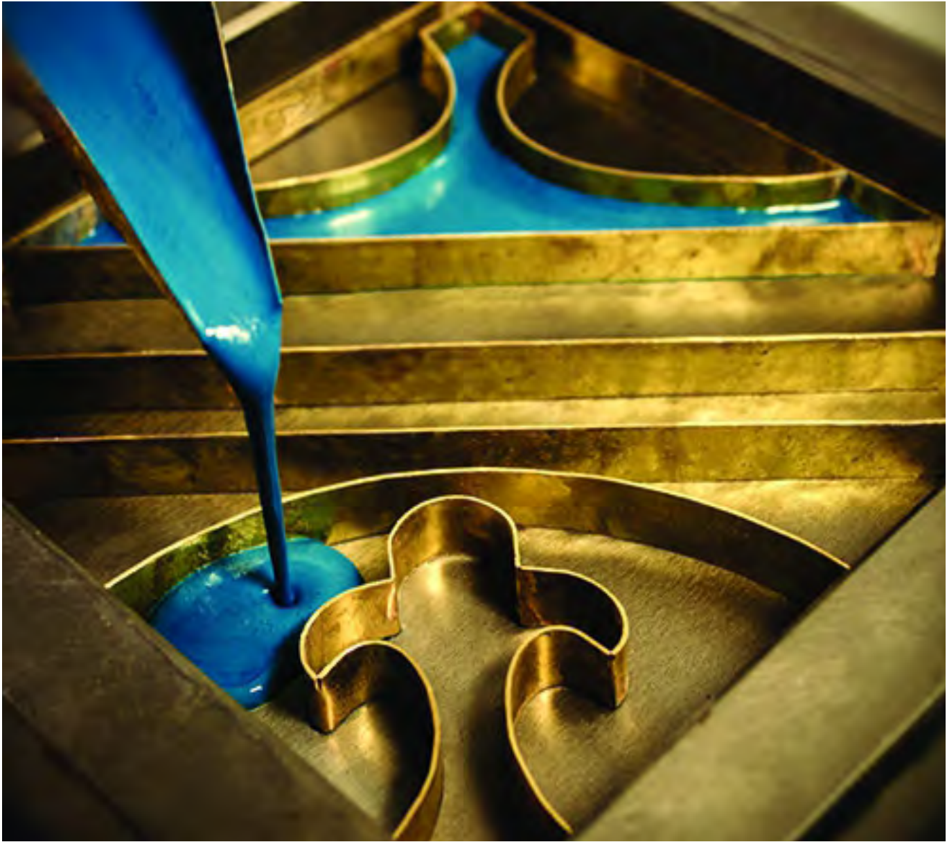
The artisans pour into a mold a mixture of pigments, ce- ment and marble powder. They work each pattern with a brass divider, like a stencil, applying each color by hand.
